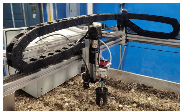
FIGURE 14. Agaricus bisporus picking robot.
