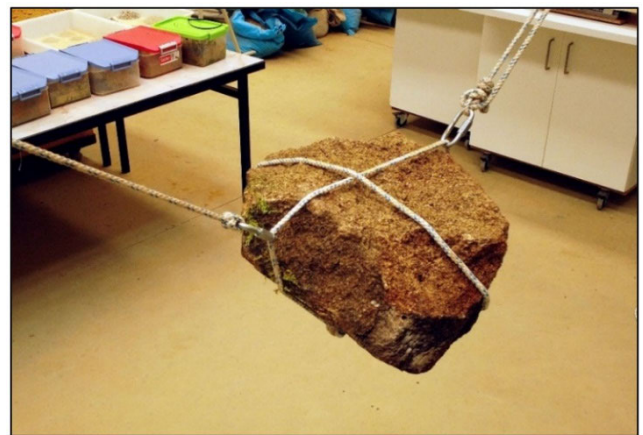
FIGURE 1. Test specimen lifted by the rope system.
