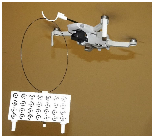
FIGURE 10. UAS transporting the scaling tool at maximum flight speed: only a slight swaying of the load is perceptible.
