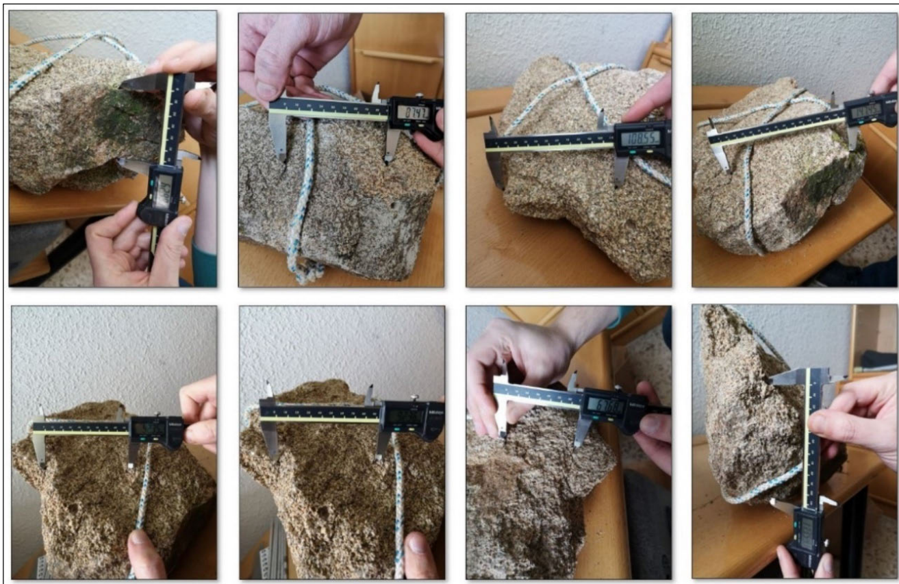
FIGURE 15. Some of the manual measurements carried out on singular points of the test specimen.
