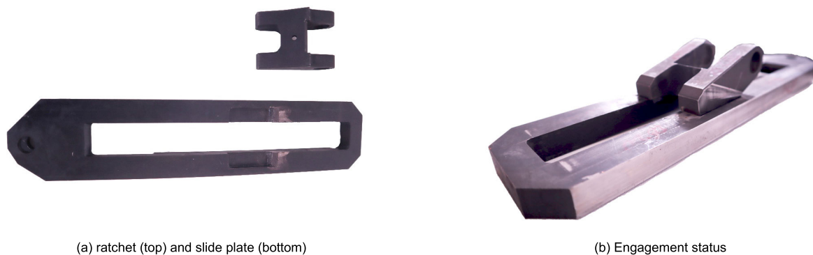
FIGURE 17. Ratchet and slide plate and its engagement relationship.
