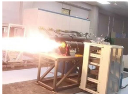
FIGURE 13. The moment the armature is discharged.
