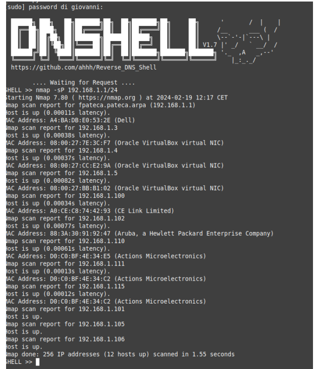
FIGURE 4. Detail of the output obtained by launching the NMap command into the DNShell.
