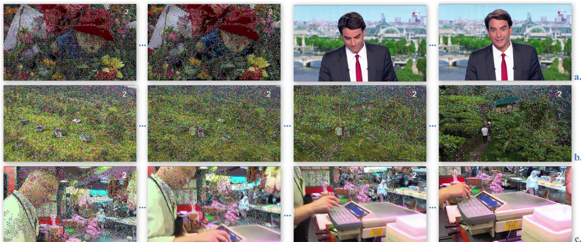
FIGURE 2. Video segmentation into shots based on interest points' analysis: (a) CUT transition; (b) Dissolve transition; (c) A video shot exhibiting important camera motion.
