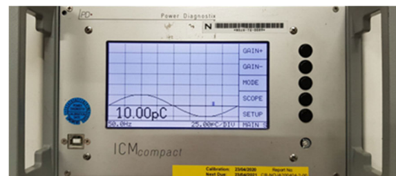
FIGURE 4. Measurement of the applied 10 pC current pulse on the display panel of the PD test set (ICMcompact - Power diagnostix systems). The yellow calibration sticker shows that the test was calibrated on 23/04/2020 and the next calibration is due on 23/04/2021. The data was collected in the mid of June 2020.
