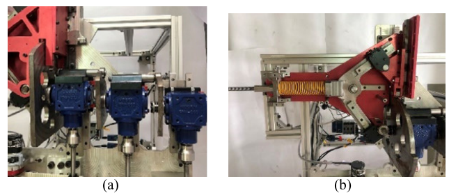
FIGURE 11. Close-up picture of the mechanism. (a) Cam series. (b) Square root mechanism.
