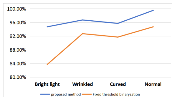
FIGURE 11. The comparison results between multi-threshold and single-threshold methods under different scenarios.
