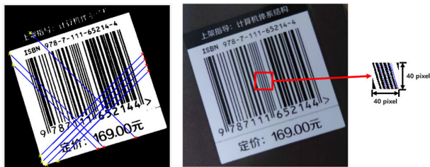
FIGURE 8. Untrimmed line detection (Left) Line detection after cropping (Right).
