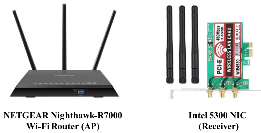
FIGURE 3. The AP and Intel 5300 NIC are used to transmit and receive Wi-Fi packets.
