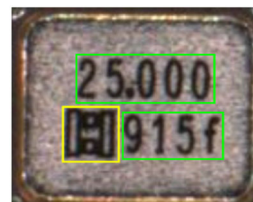
FIGURE 4. Text markings (Green box) and non-text markings (Yellow box) that are printed on a PCB component.
