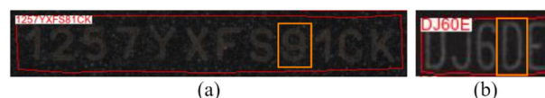
FIGURE 13. Examples of failure cases for real PCB component test images. (a) Digit “9” is predicted as “8”. (b) Alphabet “D” is predicted as digit “0”.
