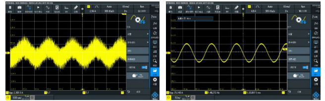
FIGURE 10. Current curve versus time when n = 750\text{rpm} . (a) Classical PID control strategy; (b) Frequency feedforward parameter compensation PID control strategy.
