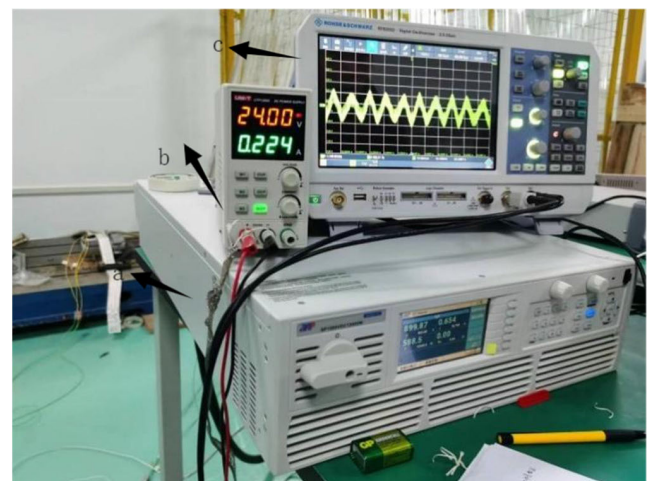
FIGURE 4. Experimental platform (Power supply and test). (a). main power, (b). auxiliary power, c. digital oscilloscope.
