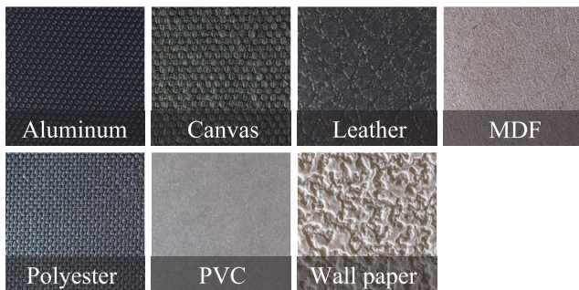
FIGURE 2. Seven texture samples used for validation. Each sample has different physical properties and was used to evaluate the texture reproduction methods in this paper. Surface images were taken with a Nikon Z6 lens (TAMRON SP AF90 mm F/2.8 Di MACRO1:1). The captured images were cropped to 15 mm in height and width.
