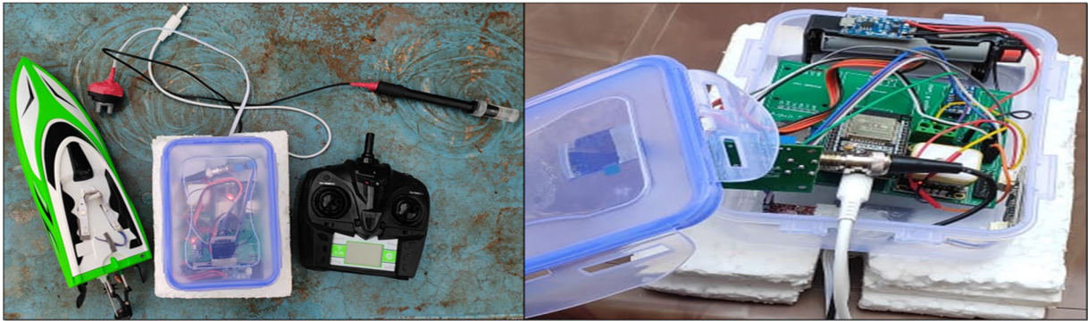
FIGURE 3. Proposed water quality monitoring system.
