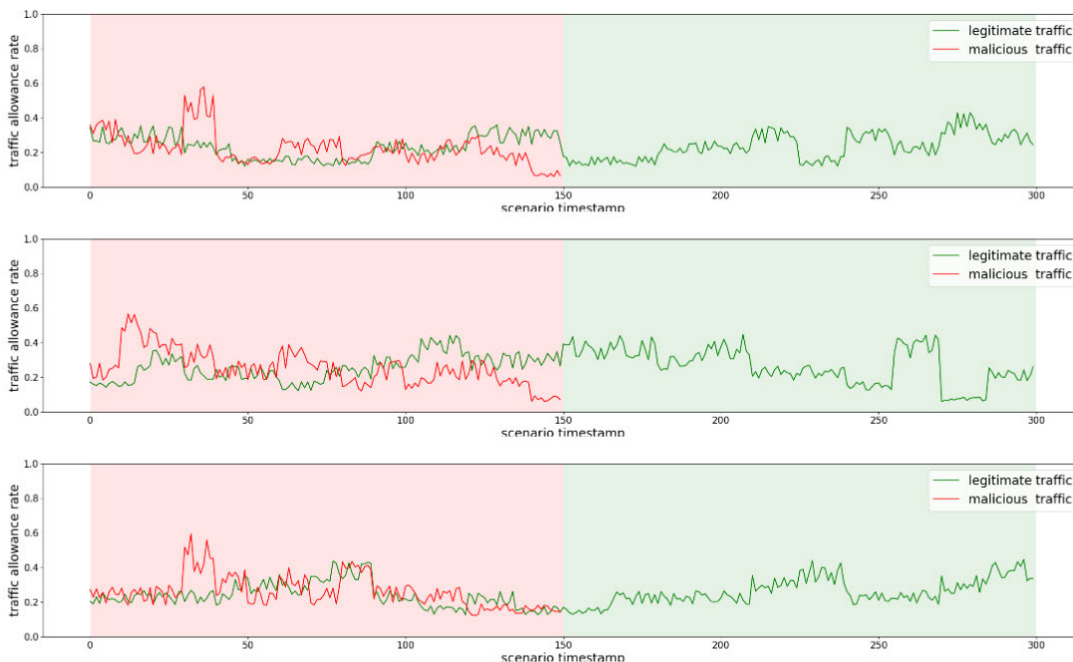
FIGURE 9. Examples of control results based on the DeepSVDD reward function in supplementary scenarios.
