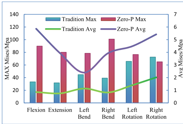
FIGURE 23. Comparison of stress value curves of two types of internal fixation screws.
