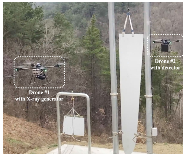
FIGURE 6. An experiment with the drone and X-ray device prototypes.
