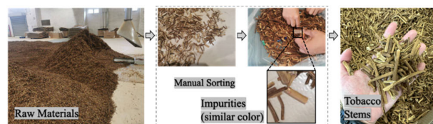
FIGURE 1. The image depicts the traditional manual sorting process in a tobacco factory, where workers separate impurities from tobacco stems by hand.
