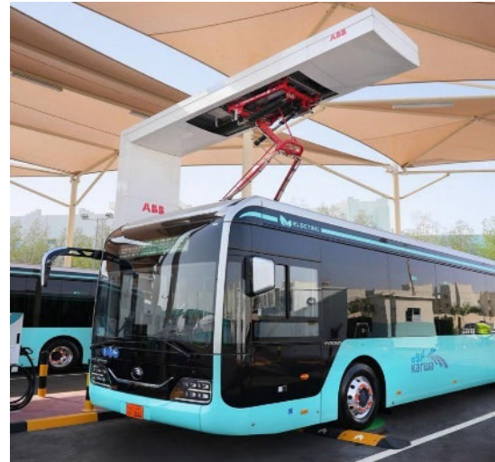
FIGURE 4. Example of top-down pantograph – Qatar [33].
