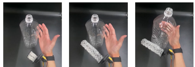
FIGURE 18. Large object grasping task (Max grasping force: 1.06[N]). A 12-layer small-sized twisted tower with a diameter of 39 mm and a height of 180 mm. The device is attached near the wrist and used to grasp a large object with one hand.
