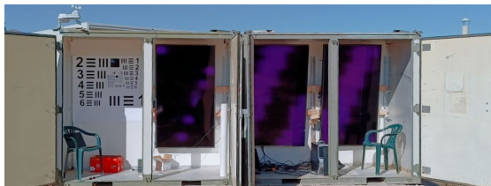
FIGURE 4. 3 × 75" 4k OLED 2,000 nit outdoor displays mounted in containers for recapture.
