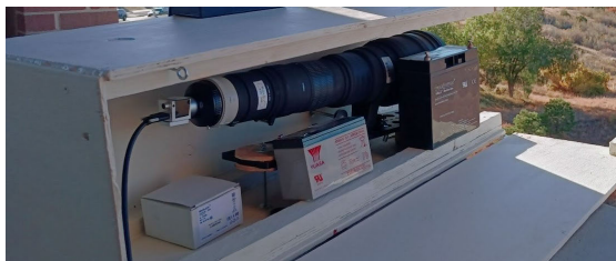
FIGURE 5. Lens and camera with custom mounting hardware for recapture.
