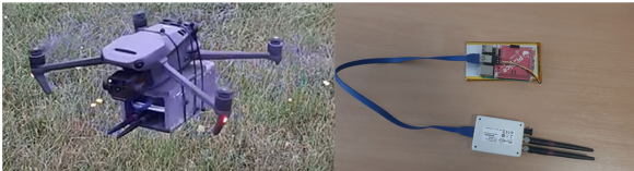
FIGURE 10. Real photo of the integrated UAV RF jammer: DJI Mavic 3 + USRP B200mini + RaspberryPi 4.
