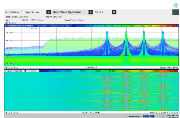
FIGURE 5. Effective jamming - an example of a narrowband jamming signal.
