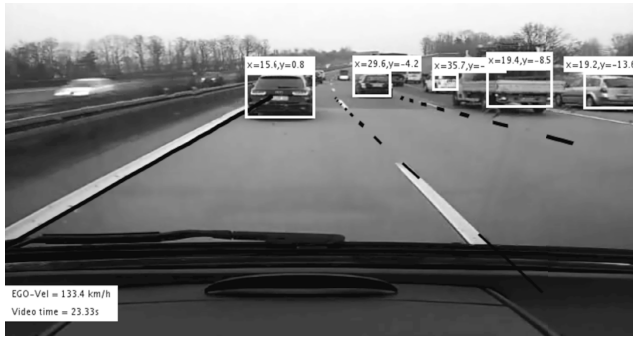
FIGURE 4. Example for a road user based view. In addition, other road users are marked with bounding boxes. Image by [83].
