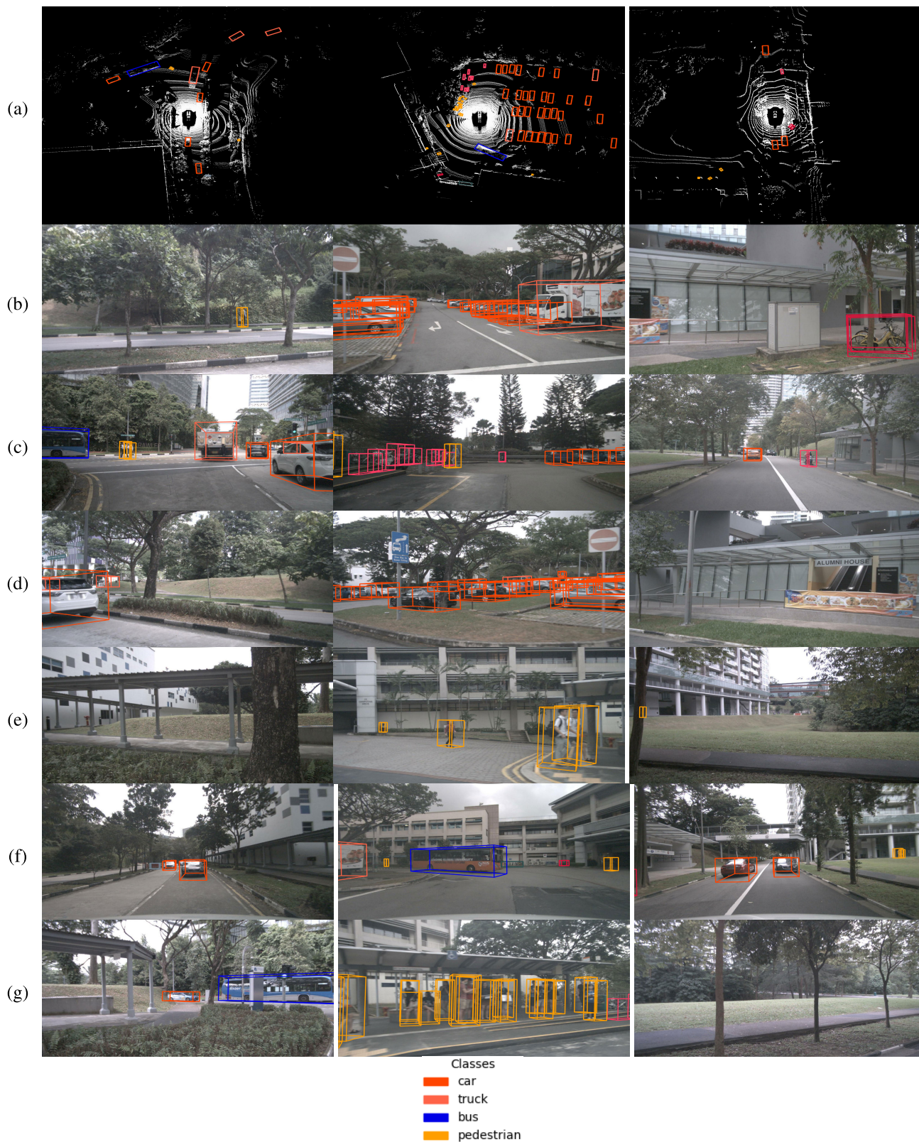
FIGURE 5. Qualitative output of 3D object detection on the nuScenes dataset. (a) BEV multimodality, (b) front left camera, (c) front camera, (d) front right camera, (e) back left camera, (f) back camera and (g) back right camera.
