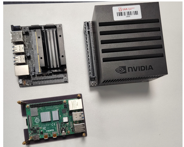
FIGURE 8. Edge computing devices used to calculate inference times for model performance. In Figure a) Nvidia Jetson Nano (top left), b) Raspberry Pi4 (bottom left), and c) Nvidia AGX Xavier (top right).
