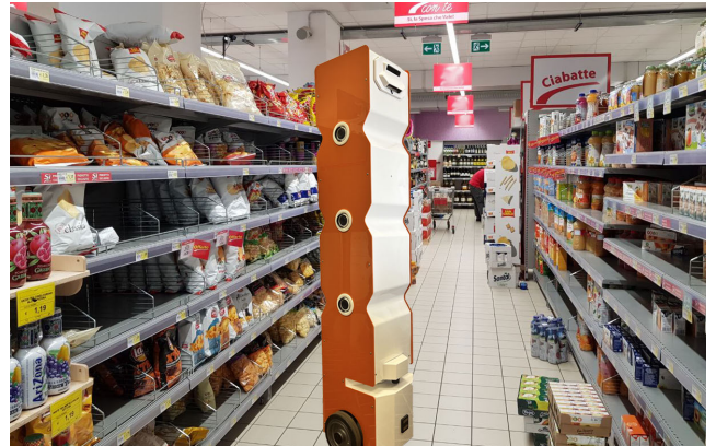
FIGURE 3. The inventory robot StockBot used for optimizing retail path planning in real environment.
