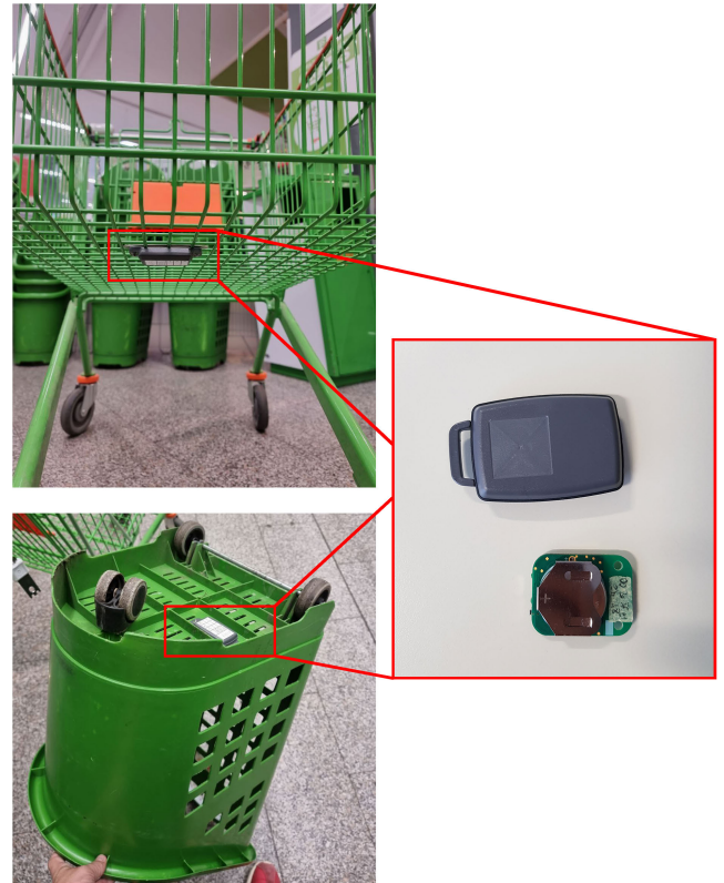
FIGURE 1. UWB tag mounted on a shopping cart and basket.
