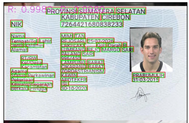
FIGURE 24. Example of the bounding box prediction from the proposed model of Indonesian ID Card with synthetic images. The green one represents the prediction bounding box and the red one represent the ground-truth bounding box.
