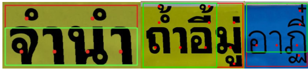
FIGURE 7. In the example images, there are the red dots appear upper and lower from the normal line. This assure that if the word has the upper or lower component, we can count the score accurately. The red boxes show the ground-truth annotation, the green boxes show the prediction result from the detection model.
