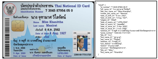
FIGURE 29. Response from Thai ID card front side pipeline. The left is the image, and the right is the response of key and value in JSON format.
