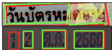
FIGURE 15. The model's predictions are represented by green boxes, while the actual ground-truth boxes are red boxes. The red dot within a box, approximates the character's position. In the above figure, it is a missing character case. There are some dots that do not intersect with the green boxes. The TedEval will count as a missing character. In the below figure, it is a missing single character case. In the first red box, there is no overlap with any green boxes, the TedEval will count as a missing single character and also count as missing character too.
