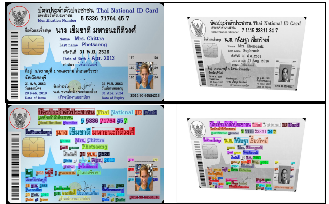
FIGURE 12. Examples of synthetic Thai ID card with ground truth COCO-instance annotation in normal cases (on the left) and augmented cases (on the right). The top upper rows are synthetic images and the bottom rows are ground-truth annotations in word-level ground-truth. And the box filled with color is the character-level ground-truth.
