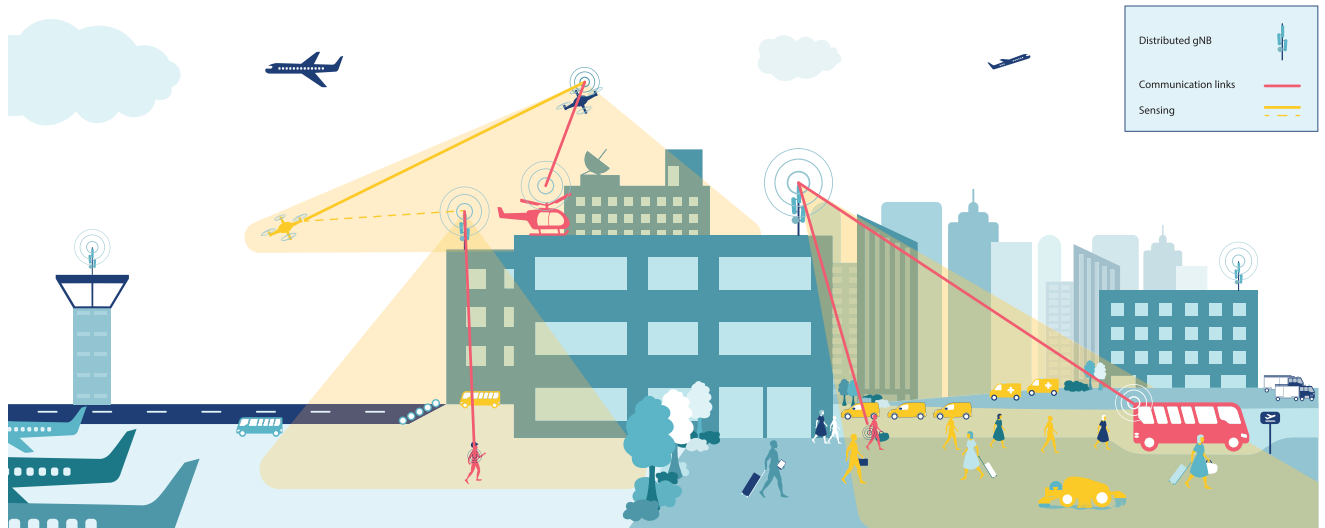
FIGURE 5. Use case for network-only JRC sensing: UAV detection and object tracking for critical infrastructure (here, an airport). Yellow lines correspond to illumination (solid) and echo (dashed) signals. Objects' and lines' colors have the same meaning as in the abstract architectural figures. Pale yellow beams depict target illumination by infrastructure nodes, capable of both communications and radar functionalities. Illuminated targets are shown in yellow colour. Notice two types of drones: one (blue) belongs to the infrastructure, acting as a mobile node capable of communications and target illumination, and another one, non-collaborative and potentially malicious, detected by the BS as a passive object. This procedure belongs to the subcategory of infrastructure-assisted JRC.
