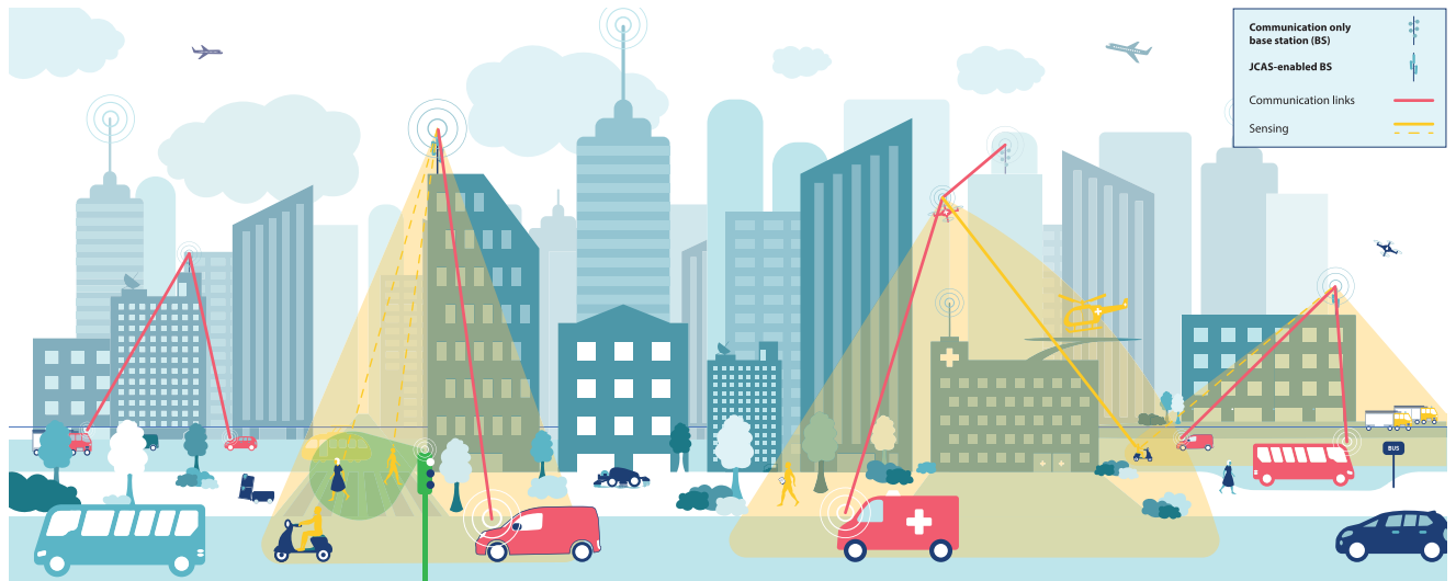
FIGURE 9. A heterogeneous JRC networks architecture consists of JRC-capable infrastructure nodes, JRC-capable UE nodes, communications-only BSs, and radar nodes. In this figure, we present a smart city scenario where nodes with different capabilities, such as JRC, communications, and sensing would coexist. JRC-capable BSs can communicate with their users (shown by the red lines) while also performing radar-based sensing operations (represented by the yellow lines). In some cases, two BSs can synchronize to conduct bistatic sensing for passive object identification, where one BS transmits its sensing signal (shown as a yellow solid line) and the other BS detects the sensing echo signal (yellow dashed line). Further, the radar-only nodes can perform their monostatic sensing operation (represented by a green beam) for passive target detection. Since all the sensing and communications operations are performed independently, all nodes can collaborate and synchronize to fuse their individual information to achieve complete and accurate sensing of the complex environment.
