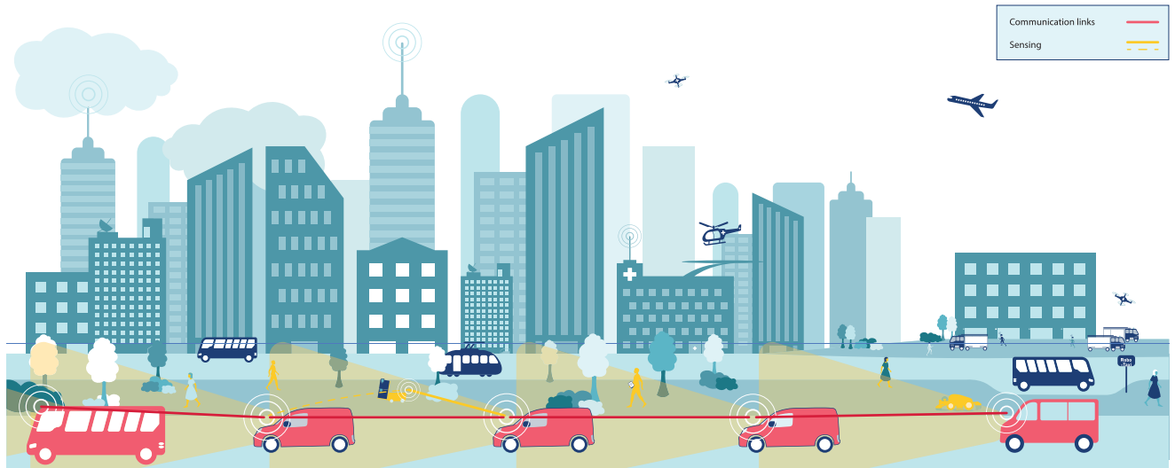
FIGURE 7. Use case for infrastructure-less JRC architecture: platooning in a city scenario with no infrastructure involved. Cars grouped together sense the environment (including group members and relevant surroundings) and share obtained information with each other, thus extending their ego view. Here, radar sensing can be performed in both mono- and bistatic modes. Passive objects to be sensed are colored in yellow. Yellow arrows represent the propagation paths of a signal used for radar purposes. Communications links are shown in red.
