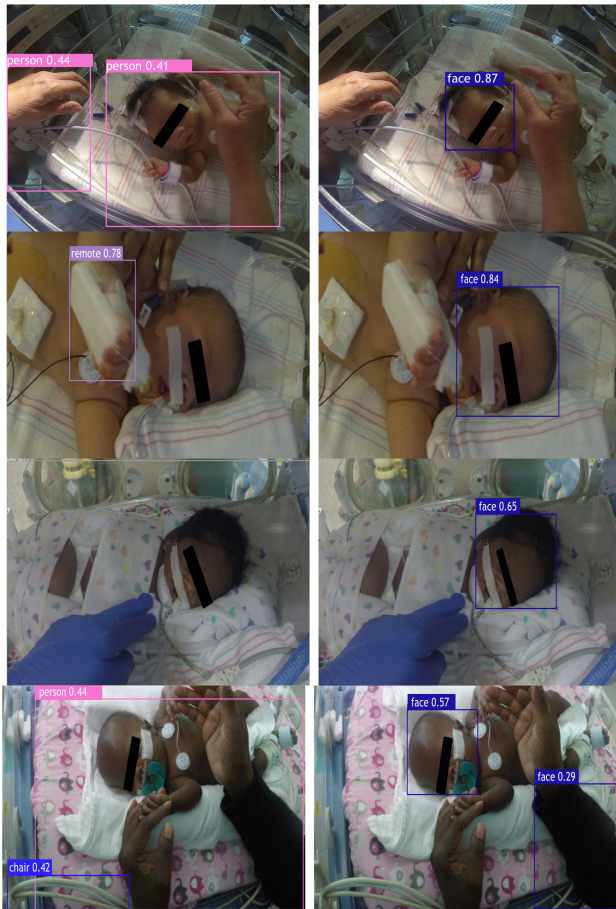
FIGURE 4. Comparison of not trained (Left Column) and trained YOLO output (Right Column).
