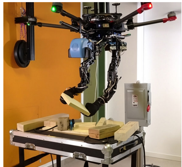
FIGURE 1. Prototype of the aerial platform used for aerial teleoperation. It is composed of a DJI hexacopter base, two 5-DoF arms based on novel soft articulated joints, two SoftHands (derivation of the PISA/IIT SoftHand [26]), and a 2-DoF head.
