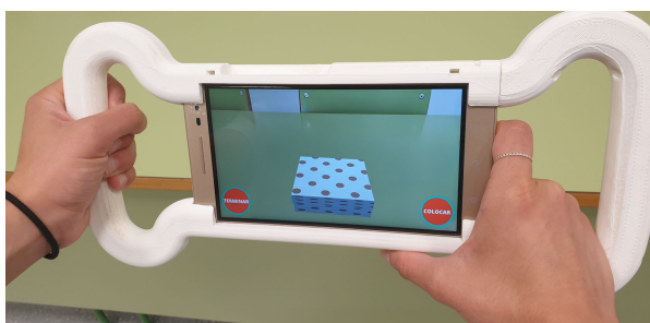
FIGURE 2. Placement of a virtual box in the desired location in the environment using the AR application.
