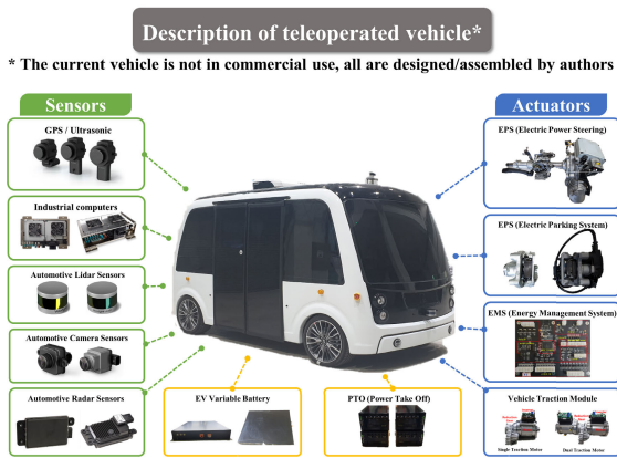
FIGURE 7. Description of the teleoperated vehicle used in the experiment.
