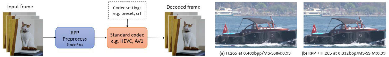
FIGURE 5. Preprocessing in video showing the deployment workflow of the rate-perception optimized preprocessor (RPP) and a comparison of frame segments of H.265 and RPP + H.265 at the same MS-SSIM, [26].
