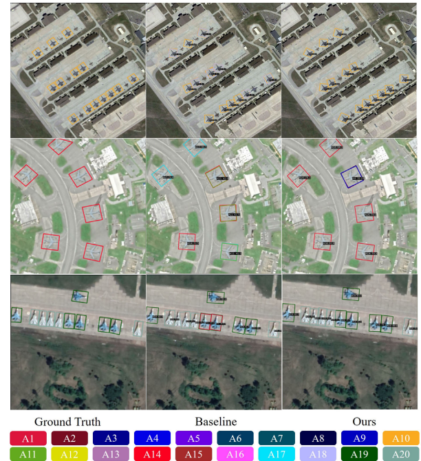
FIGURE 6. The depicted image demonstrates the outcomes derived from our proposed approach on the MAR20 dataset, encompassing 20 distinct categories. The initial column portrays the dataset's authentic annotations, while the second column displays the baseline results, and the third column exhibits our method's outcomes. Each row corresponds to three sets of results for a single image. The rectangular boxes labeled A1 to A20 at the bottom signify the distinct colors representing respective category bounding boxes.
