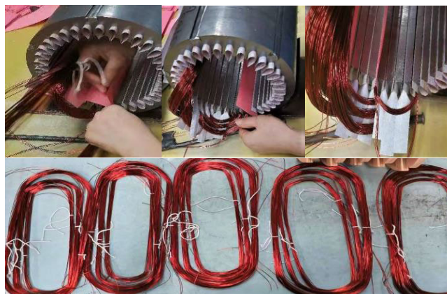
FIGURE 9. Concentric unequal turns winding and embedding process.
