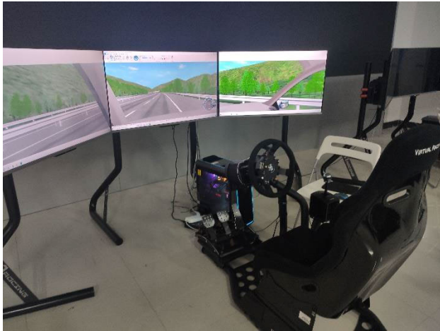
FIGURE 3. Driving simulation equipment.
