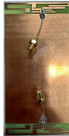
FIGURE 22. A photo of the 2 × 2 MIMO antenna system on the all-metal backplane of a smartphone.
