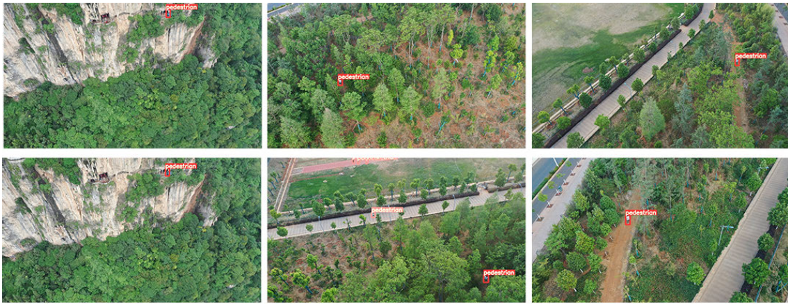
FIGURE 6. Target detection is performed for targets in remote sensing images taken at different locations at the same moment, and the correspondence between targets is established using the ReID method. The two images in the same column are images of the same set of different locations taken at the same time, and we have marked the same targets with the same color for identification. More obvious is the second set of images, where the red anchor box is the corresponding target after re-identification, and the pink is the target not found in the corresponding figure.
