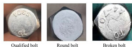
FIGURE 1. Some surface defects of metal components.
