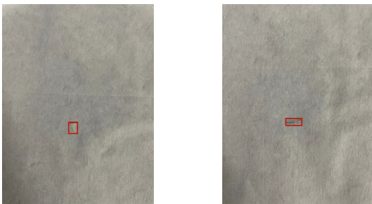
FIGURE 2. Blemishes similar to the background.
