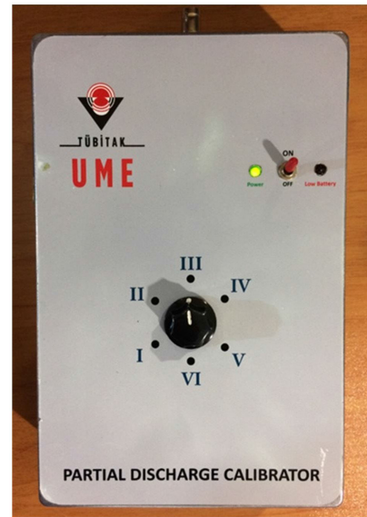
FIGURE 10. The industrial partial discharge calibrator (TÜBITAK UME).
