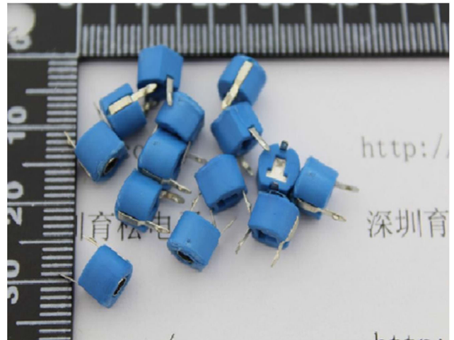
FIGURE 6. Adjustable capacitors used in the production of PD pulses.
