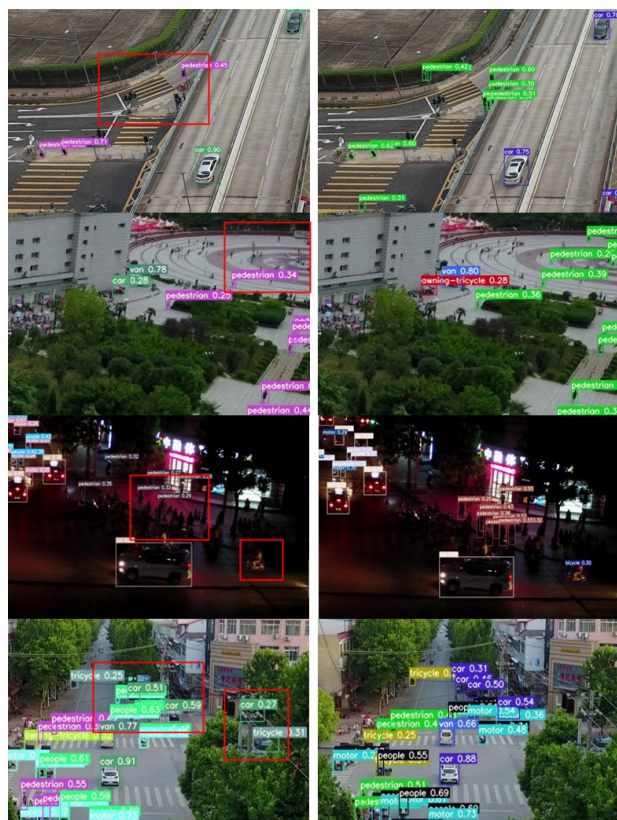
FIGURE 7. Comparison of YOLOv7 and MCA-YOLOv7 detection effect. The YOLOv7 detection result is on the left, while the MCA-YOLOv7 result is on the right. It is evident that, in comparison to the left, the right has a lower false and missed detection rate.
