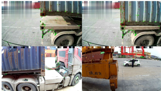
FIGURE 11. Key-points (green dots) within entire images. There are many useless and even interfering key-points. It is challenging to identify which object each key-point belongs to, whether the truck is present, where the truck body is, and whether the truck is lifted.
