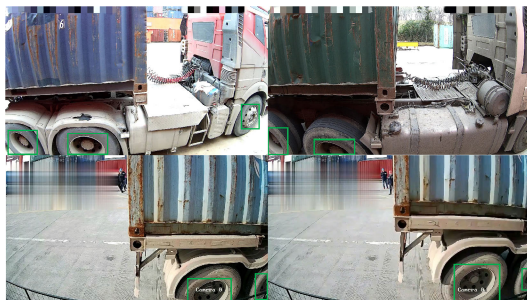
FIGURE 13. Wheel hubs detection results of the method in [9] in our scenario. The green rectangles represent the approximate regions of wheel hubs detected by the first-stage object detector in [9], while the Hough circle detector, i.e., the second-stage detector in [9], fails to further locate the wheel hubs.
