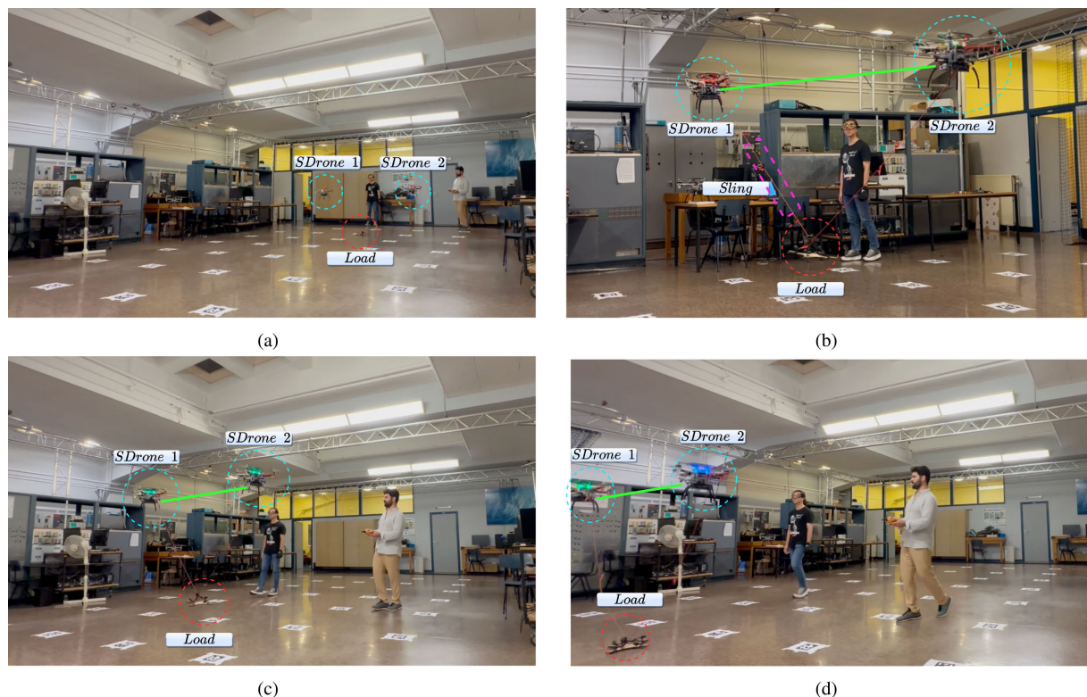
FIGURE 10. Demonstration of multi-UAV object transport: (a) Coordinated take-off. (b) UAVs navigating the environment. (c) Arrival at the target destination. (d) Coordinated descent ensuring safe payload placement.
