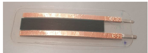
FIGURE 4. OPV based on LAYER® technology. Fabricated by Dracula Technologies.
