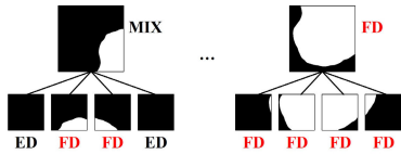
(b) Generating the state value of parent nodes in a bottom-up manner
