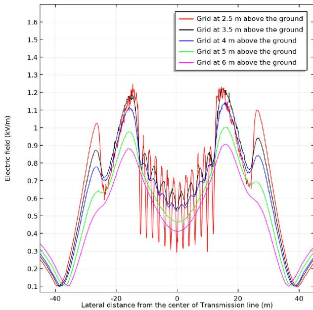
**FIGURE 5.** The effect of the shielding grid height from the ground level on the electric field intensity at level 1.8 m above the ground.
