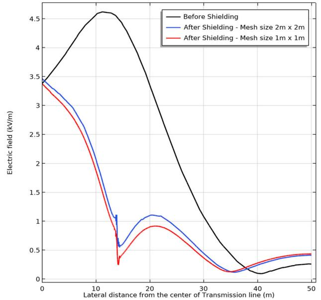
FIGURE 14. The effect of the mesh dimensions on both the distribution and reduction of the electric field.
