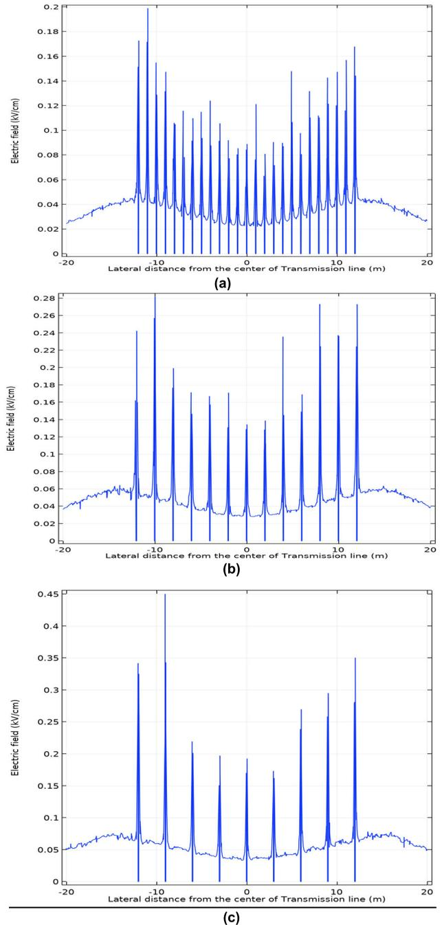
**FIGURE 6.** The Electric field intensity at the grid level of 6 m above the ground using different grid mesh sizes: (a) grid mesh sizes of 1 × 1 m (safe), (b) grid mesh sizes of 2 × 2 m (safe), and (c) grid mesh sizes of 3 × 3 m (safe).
