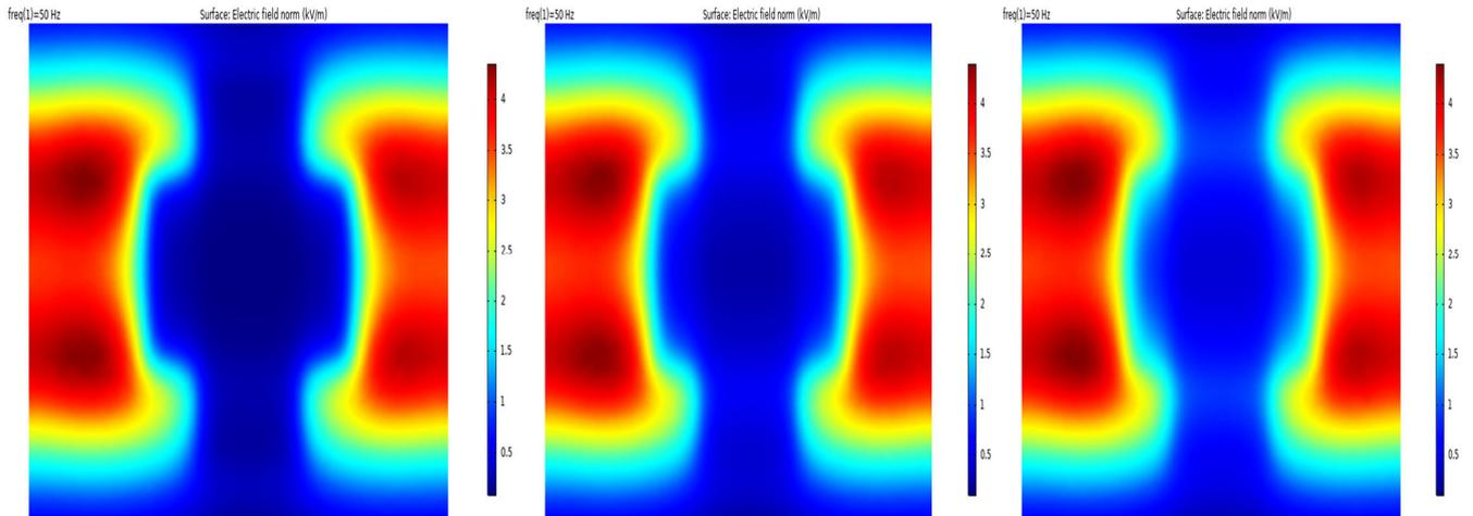
**FIGURE 9.** Maps of the electric field density under the zone covered by the earthed shielding grids: (a) grid mesh of 1 × 1 m dimensions, (b) grid mesh of 2 × 2 m dimensions, and (c) grid mesh of 3 × 3 m dimensions.
