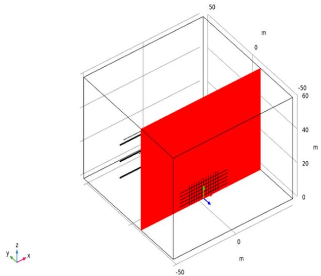
**FIGURE 11.** Simulation of the grounding grid installed beside the high-voltage line.
