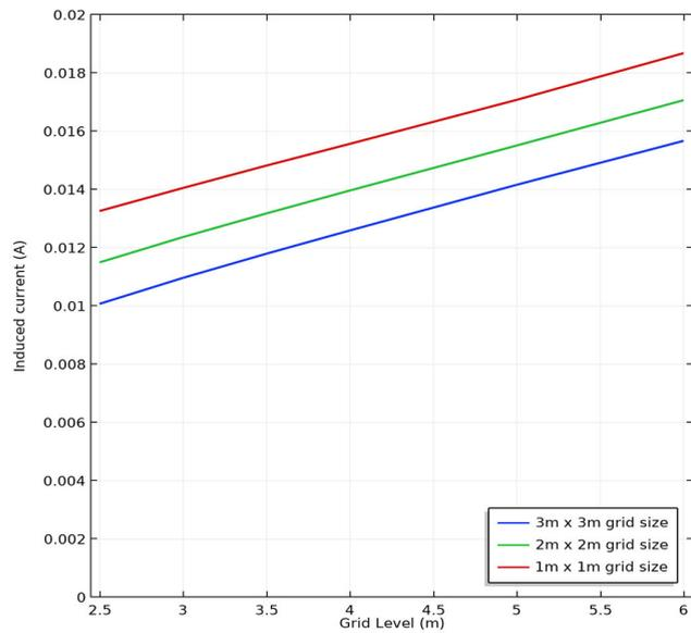
**FIGURE 10.** The capacitive current between the transmission line conductors and the installed earthed shielding grids.
