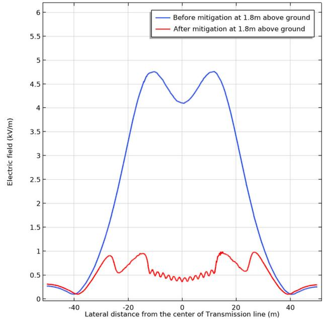
FIGURE 4. The electric field intensity at 1.8 m level without and with earthed shielding grid.
