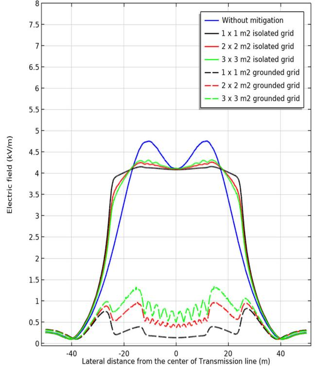
**FIGURE 8. Comparison between the isolated and earthed grids with different mesh dimensions.**
