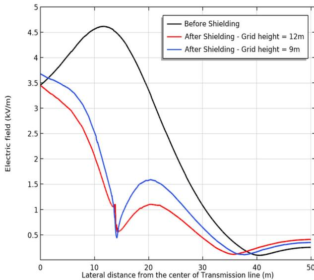
FIGURE 13. The Impact of the earthed shielding grid height beside and parallel to the lines on the distribution of the electric field near the lines (2m x 2m grid dimensions case).
