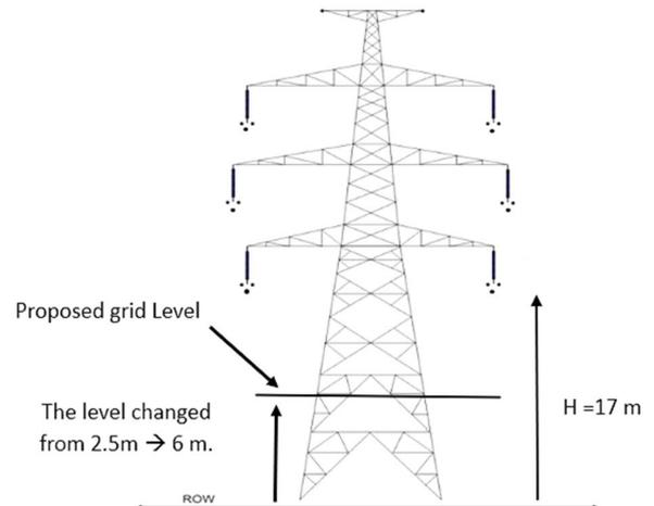
FIGURE 2. 500 kV double circuits EHVTL, 3 bundles per phase.
