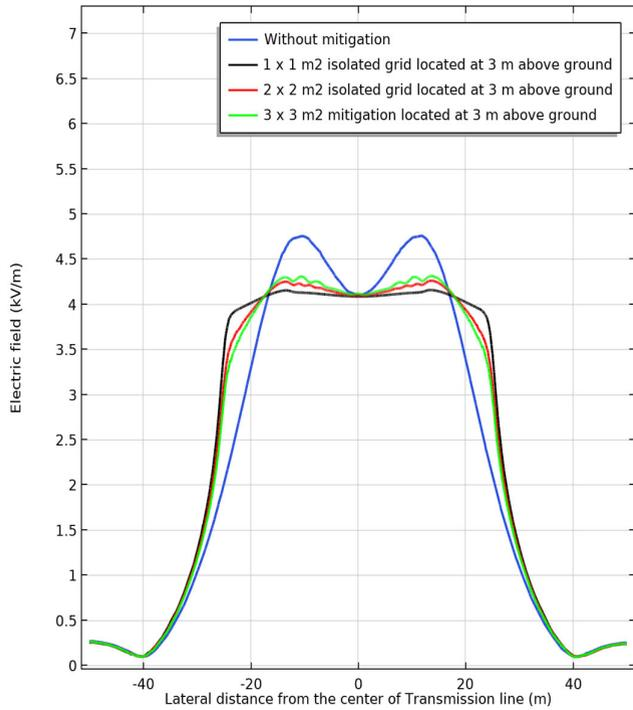
**FIGURE 7. Electric field with isolated grid using different mesh dimensions.**
