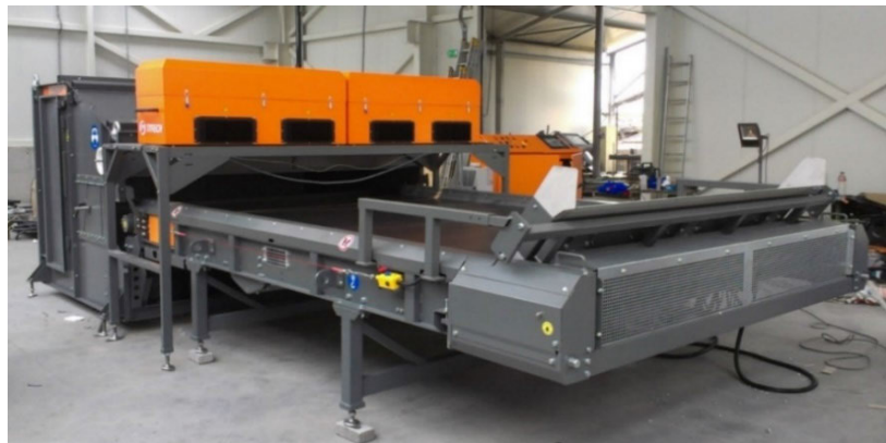
FIGURE 3. Line with NIR/VIS optical sorting system.
