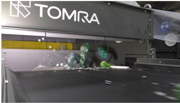
FIGURE 5. Schematic of the detection and ejection of plastic waste on the NIR/VIS optical sorting system.
