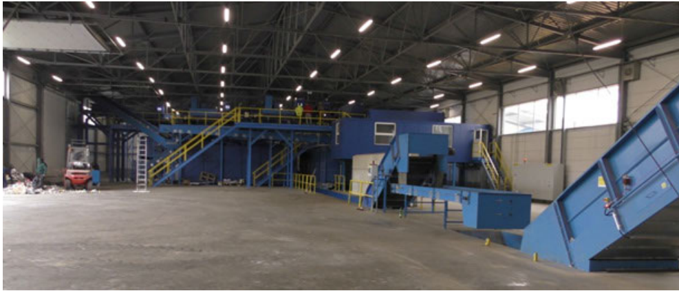
FIGURE 2. The complete sorting line in the production hall.
