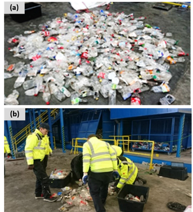
FIGURE 16. (a) Sample of sorted waste, (b) manual removal of contamination.
