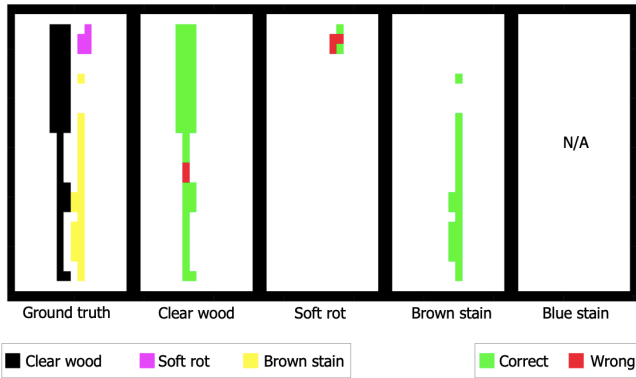
FIGURE 3. Example of classification map produced by the end-to-end framework on a sample HSI wood board of size 897 \times 512 \times 337 .
