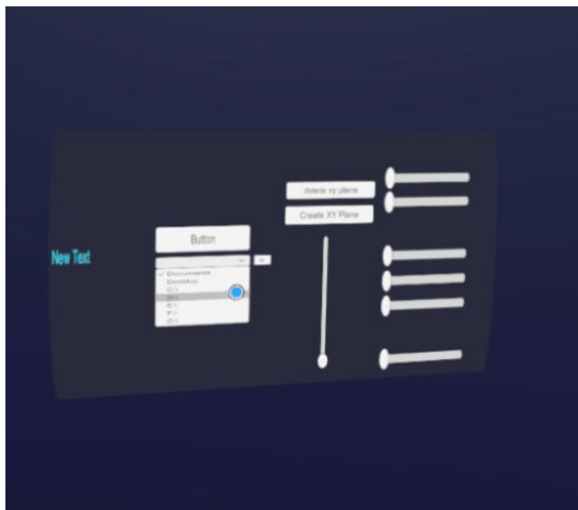
FIGURE 5. File browser component in a VR environment allows users to select DICOM data directories. The image showcases the file browser component, presented as a drop-down menu within the VR environment.
